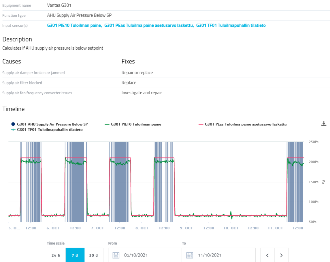
Figure 26: An example of different analytics performed in Caverion SmartView.
